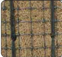
Created with three UV-stabilized nets, the three dimensional TRM will provide protection through all phases of vegetation growth. The layer of coconut fiber is slow to degrade and helps with the germination. This is an excellent choice for high-flow areas and steep embankments where a permanent solution is needed
