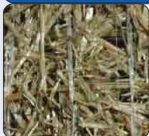
Designed to provide erosion protection up to 45-90 days, it can be used in areas up to a 2:1 slope that requires quick mowing. The double netting ensures more efficient erosion protection and plant growth than the single layer of netting.
