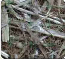
Engineered for erosion protection for up to 24 months, the ECSC-2 is designed for use in moderate-heavy flow channels and on slopes up to a 1:1 grade. The combination of the two effective matrixes provides extra protection for extended vegetation growth.
