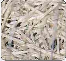
Designed for areas with moderate flow channels and slopes up to 2:1, the erosion blanket will provide protection for 12 months. Made with 100% Aspen wood fiber, the matrix will enhance water absorption, therefore aiding in quicker vegetation establishment.
