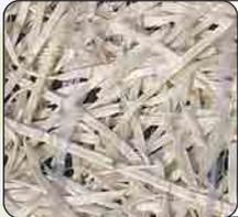
Designed for areas with moderate flow channels and slopes up to 1.5:1 the erosion blanket will provide protection for 24 months. Made with 100% Aspen wood fiber, the matrix will enhance water absorption, therefore aiding in quicker vegetation establishment. The double netting provides more stability over the single net.
