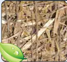
Made with a blend of straw and coconut, the ECSC-2B offers protection up to 18 months and works effectively in moderate flow rainfall and runoffs, and on slopes up to 1:1 grade. The addition of coconut to the straw increases the absorption amount and provides extra protection for extended vegetation growth.
