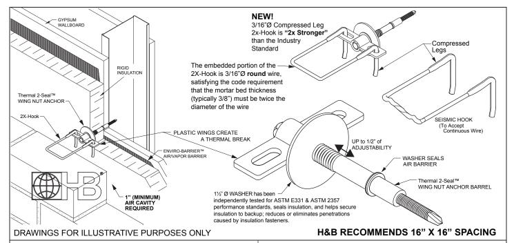
Hohmann & Barnard's 2X-Hook has been tested and designed to withstand over 200-lbf, in tension or compression, at maximum allowed offset (ACI 530 6.2.2.5.5.4) of 11/4". These results exceed BIA recommendations and the capabilities of standard "round wire" hooks/pintles by over 100%, creating a higher standard for the masonry industry. Test results available upon request. 2X-Hook: U.S. Pat. No. 8,613,175
