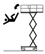
ALWAYS USE 'THREE POINT CONTACT' WITH THE MACHINE. FACE THE MACHINE WHEN ENTERING OR LEAVING THE PLATFORM. 'THREE POINT CONTACT' MEANS THAT TWO HANDS AND ONE FOOT OR ONE HAND AND TWO FEET ARE IN CONTACT WITH THE MACHINE AT ALL TIMES DURING MOUNT AND DISMOUNT.
