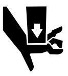
NEVER WORK UNDER AN ELEVATED PLATFORM UNTIL IT HAS BEEN RESTRAINED FROM MOVEMENT WITH SAFETY PROPS, BLOCKING OR OVERHEAD SLING.
