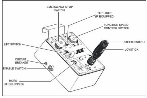
Figure 3-2. Platform Control Station
