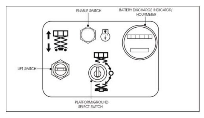
Figure 3-1. Ground Control Station
