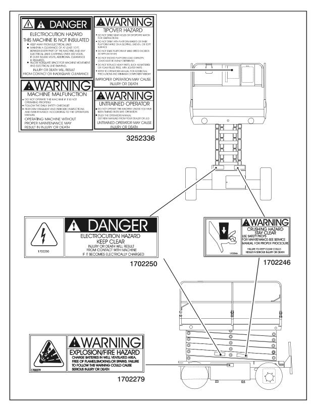
Figure 3-5. Decal Location (left side and front)
